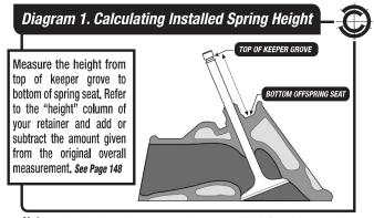
*Note:* If heads have been extensively modified (machined spring pockets, longer valves, etc.) contact Crower for proper spring, keeper, cup and retainer recommendations. Have your keeper/seat measurement available.
